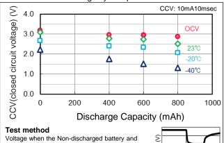
voltage when the Non-discharged battery and the battery discharged to the specific capacity(400mAh,600mAh,800mAh @23°C,3kΩ) is measured under the condition of 10mA ×10msec (1 pulse).
