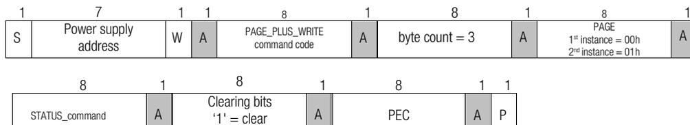
STATUS\_WORD cannot be cleared directly It is cleared based on lower-level status commands
