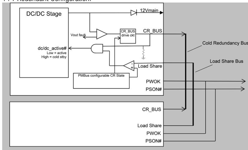
Cold Redundancy 2+2 & 3+1 Configuration:
