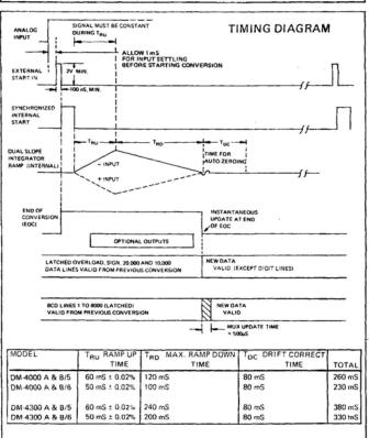
NOTE: BCD OUTPUTS NOT VALID UNTIL 500  $\mu$ SEC AFTER EOC FALLING EDGE.
