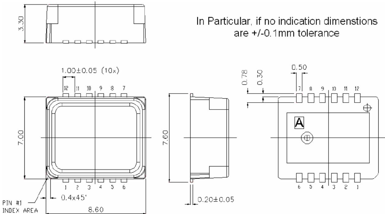
Figure 2 Outline and dimensions for 12 lead DFL package.
