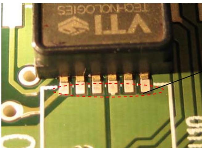
Extended land pad area, where soldering iron should touch
