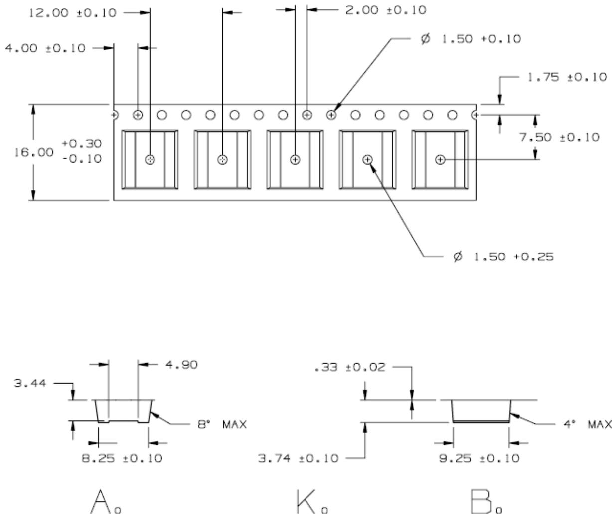
Figure 3 Packing tape dimensions for the 12 lead DFL Package. Dimensions in millimeters [mm].
