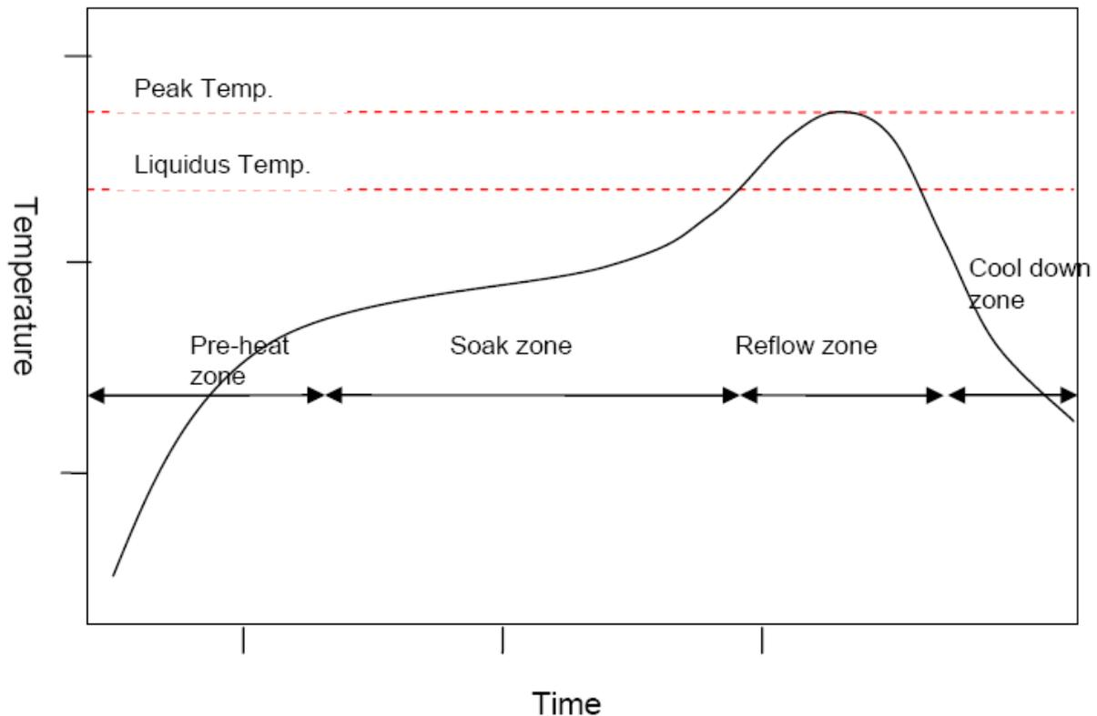
**Figure 7 Typical convection reflow soldering phases and profile.**
