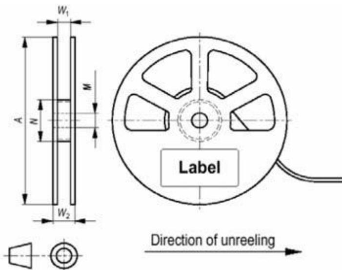
**Figure 5 Reel dimensions. All dimensions in millimeters [mm].**
