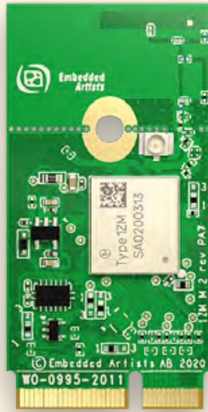
Type 1ZM Dual band Wi-Fi® 11a/b/g/n/ac + Bluetooth® 5.1
