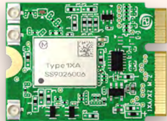
Type 1XA Dual band Wi-Fi® 11a/b/g/n/ac 2x2 MIMO / RSDB + Bluetooth® 5.2 (PCIe)
