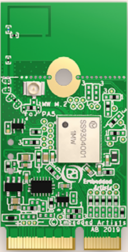
Type 1MW Dual band Wi-Fi® 11a/b/g/n/ac + Bluetooth® 5.0
