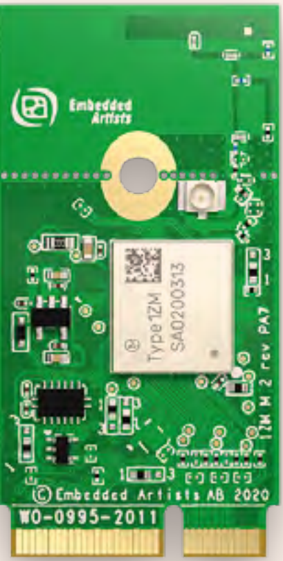
Type 1ZM Dual band Wi-Fi® 11a/b/g/n/ac + Bluetooth® 5.1
