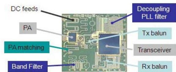
**Figure 2 - Example of 2D PICS interposer with active dies**
