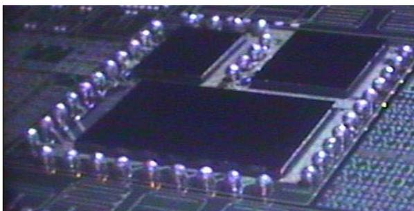
Figure 4 - Sub-system on PICS interposer
