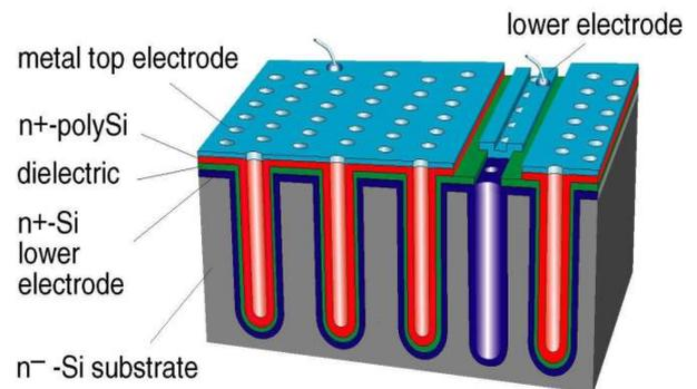
Figure 9 – Cross-sectional view of IPDiA high density capacitor
