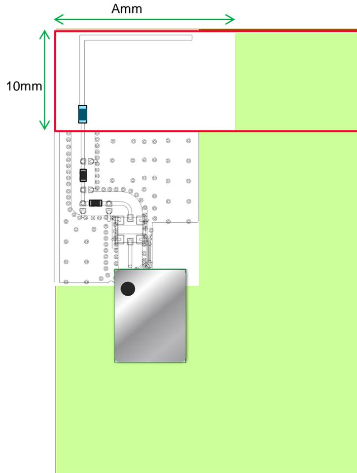
If PCB has to arrange GND plane in antenna right area
