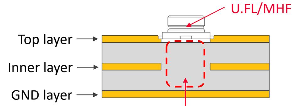
Do not place any conductors such as GND, signal traces, power lines more than 400um from bottom of the connector.
