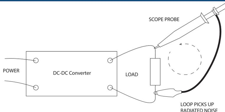
**Figure 12: CORRECT WAY TO MEASURE DIFFERENTIAL NOISE**
