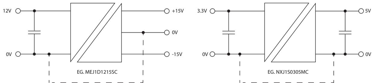
**Figure 5: CONFIGURATIONS OF ISOLATED DC-DCs PRODUCING AUXILIARY VOLTAGES**
