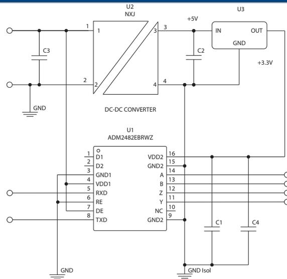
**Figure 4: TYPICAL LOW POWER DC-DC APPLICATIONS**
