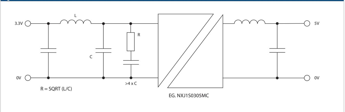
**Figure 10: INPUT COMMON MODE FILTERING**
