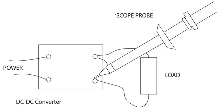
**Figure 13: OUTPUT RIPPLE AND NOISE CHARACTERISTICS**
