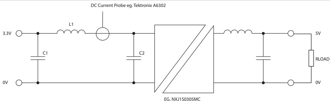
C1 - 220 $\mu$ F with ESR of <0.1 $\Omega$  at 100kHz, rated at supply voltage.
