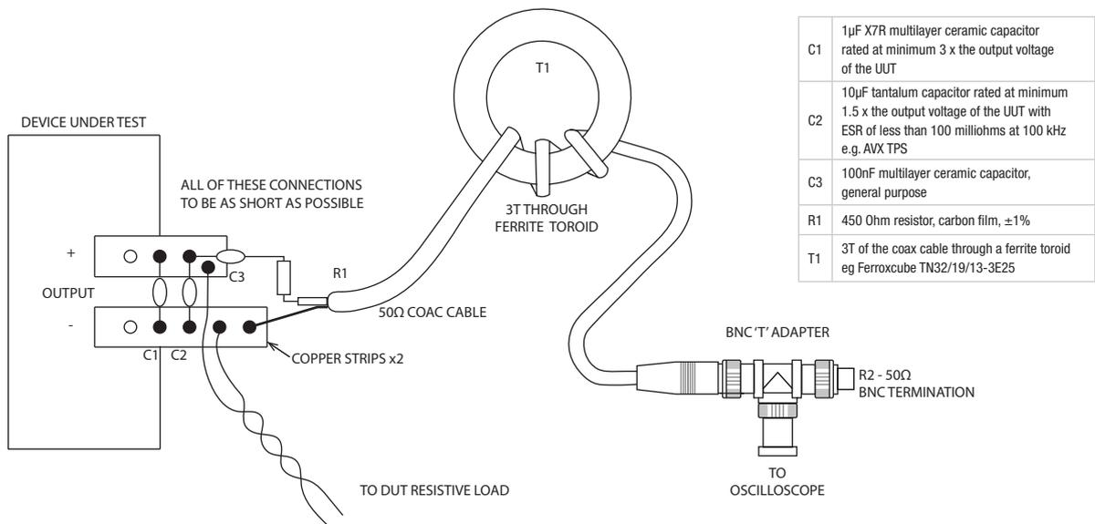
**Figure 14: STANDARDISED TEST METHOD FOR INPUT RIPPLE CURRENT**
