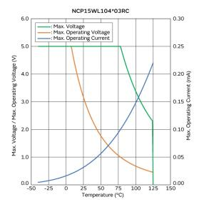
Max. Voltage, Max. Operating Voltage/Current Reduction Curve
