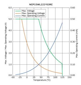
Max. Voltage, Max. Operating Voltage/Current Reduction Curve
