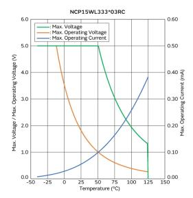
Max. Voltage, Max. Operating Voltage/Current **Reduction Curve**
