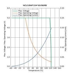
Max. Voltage, Max. Operating Voltage/Current **Reduction Curve**
