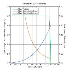
Max. Voltage, Max. Operating Voltage/Current **Reduction Curve**
