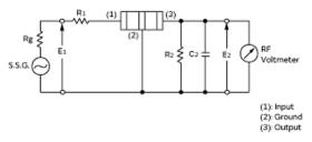
Rg = 50Ω R1 = 420Ω ±5% R2 = 470Ω ±5% C2 = 10 ± 2 pF (Including stray capacitance and Input capacitance of RF Voltmeter) E1: S.S.G. Output Voltage
