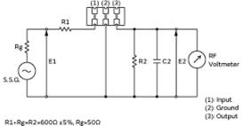
C2=10pF (including stray capacitance and input capacitance of RF Voltmeter) E1: S.S.G. Output voltage
