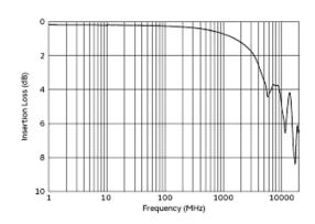
Common Mode Insertion Loss Characteristic (Typical Value)
