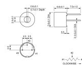
unit : mm Tolerance : ±0.3 Note: This datasheet may be out of date. Please download the latest datasheet of PV12P102A01B00 from the official website of Murata Manufacturing Co., Ltd.
