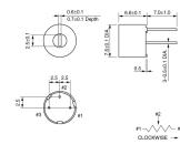
unit : mm Tolerance : ±0.3 Note: This datasheet may be out of date. Please download the latest datasheet of PV12P103A01B00 from the official website of Murata Manufacturing Co., Ltd.
