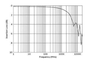
Common Mode Insertion Loss Characteristic (Typical Value)
