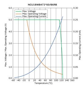
Max. Voltage, Max. Operating Voltage/Current **Reduction Curve**
