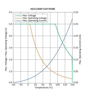
Max. Voltage, Max. Operating Voltage/Current Reduction Curve
