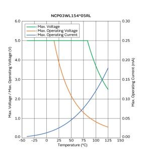
Max. Voltage, Max. Operating Voltage/Current Reduction Curve
