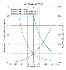
Max. Voltage, Max. Operating Voltage/Current **Reduction Curve**
