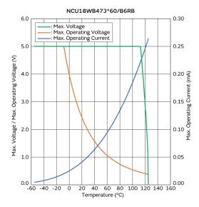
Max. Voltage, Max. Operating Voltage/Current **Reduction Curve**
