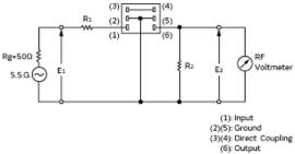
R1 + Rg = R2 =Input and Outout Impedance E1: S.S.G. Output Voltage
