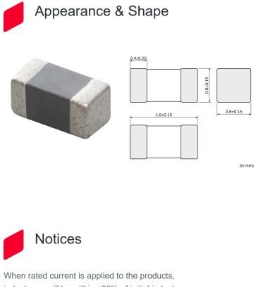
inductance will be within ±30% of initial inductance value range. When rated current is applied to the products, the temperature rise caused by selfgenerated heat shall be limited to 40°C max. Keep the temperature (ambient temperature plus selfgeneration of heat) under 125°C.
