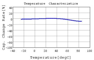
DE1B3RA681KN4APO1F C-Temp. capchange, DCOV,
