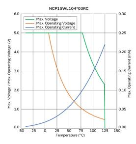
Max. Voltage, Max. Operating Voltage/Current **Reduction Curve**
