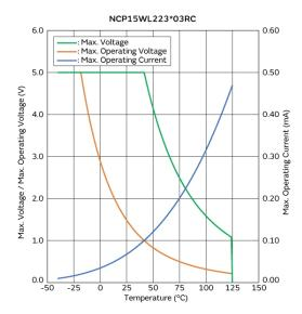
Max. Voltage, Max. Operating Voltage/Current **Reduction Curve**
