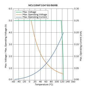
Max. Voltage, Max. Operating Voltage/Current **Reduction Curve**
