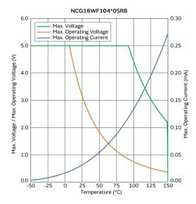
Max. Voltage, Max. Operating Voltage/Current **Reduction Curve**
