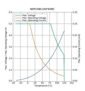
Max. Voltage, Max. Operating Voltage/Current Reduction Curve
