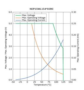
Max. Voltage, Max. Operating Voltage/Current Reduction Curve
