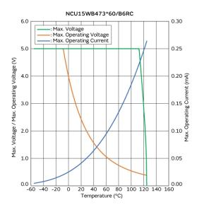
Max. Voltage, Max. Operating Voltage/Current **Reduction Curve**
