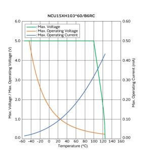
Max. Voltage, Max. Operating Voltage/Current Reduction Curve
