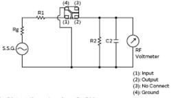
R1+Rg=R2=Input/Output Impedance, Rg=50Ω C2=10pF (Including stray capacitance and Input capacitance of RF Voltmeter) E1: S.S.G. Output Voltage
