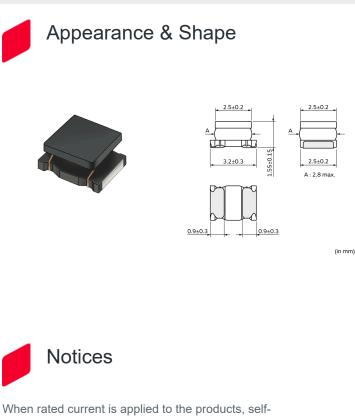
temperature rise shall be limited to 20°C max and inductance will be within ±10% of initial inductance value.
