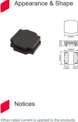
When rated current is applied to the products, inductance will be within  $\pm 30\%$  of nominal inductance value. When rated current is applied to the products, the temperature rise caused by selfgenerated heat shall be limited to 40°C max. Keep the temperature (ambient temperature plus selfgeneration of heat) under 125°C.
