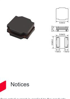
When rated current is applied to the products, inductance will be within ±30% of nominal inductance value. When rated current is applied to the products, temperature rise caused by selfgenerated heat shall be limited to 40°C max. Keep the temperature (ambient temperature plus selfgeneration of heat) under 125°C.
