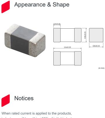
When rated current is applied to the products, inductance will be within  $\pm 30\%$  of initial inductance value range. When rated current is applied to the products, the temperature rise caused by selfgenerated heat shall be limited to 40°C max. Keep the temperature (ambient temperature plus selfgeneration of heat) under 125°C.
