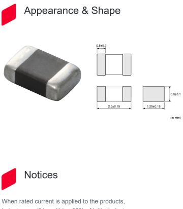
When rated current is applied to the products, inductance will be within ±30% of initial inductance value range. When rated current is applied to the products, the temperature rise caused by selfgenerated heat shall be limited to 40°C max. Keep the temperature (ambient temperature plus selfgeneration of heat) under 125°C.
