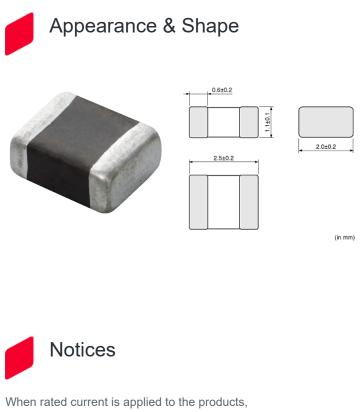
When rated current is applied to the products, inductance will be within  $\pm 30\%$  of initial inductance value range. When rated current is applied to the products, temperature rise caused by selfgenerated heat shall be limited to 40°C max. Keep the temperature of product (ambient temperature plus self-generation of heat) under 125°C.
