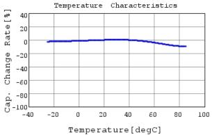
DE1B3RA331KN4APO1F C-Temp. capchange, DCOV,
