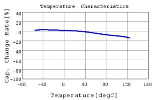
RCER71E106K3M1H03A C-Temp. capchange, DCO.ON
