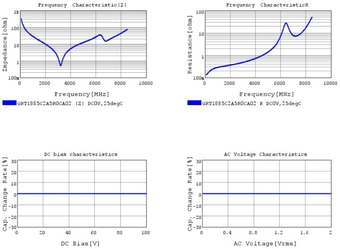
GRT1885C2A5ROCAO2 C-DC bias capchange, 25.00 GRT1885C2A5ROCAO2 C-AC Voltage capchange, DC
