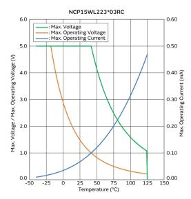
Max. Voltage, Max. Operating Voltage/Current **Reduction Curve**
