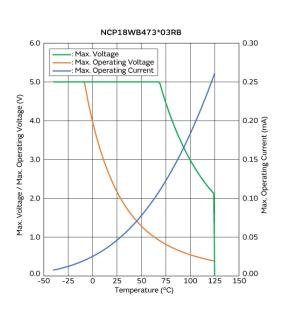
Max. Voltage, Max. Operating Voltage/Current Reduction Curve
