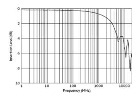
Common Mode Insertion Loss Characteristic (Typical Value)
